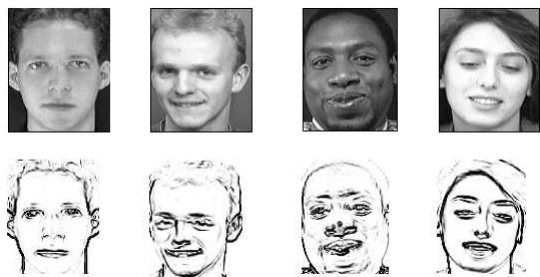
Fig. 5. Examples of Edges Detection with the Type-2 FIS method
